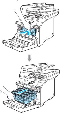
4 Release the gray lock lever (1) that is on the left side of the machine. Lift the front of the drum unit and pull the drum unit completely out of the machine using the green handles on the drum unit.
